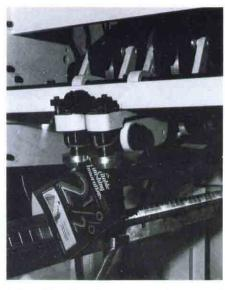
Adjustable forming rollers finish and sharpen the fold formed by the male and female conveyor belts. Fold quality and accuracy is excellent.
