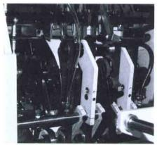
Scoring unit can be set for inside or outside surface score, whichever gives the smoothest, sharpest fold on a particular stock. Changeover from one type of score to the other can be done in just a few minutes.
