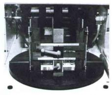
Turntable rotates 180 degrees while the next lift is formed in the upper bin. When the pre-set count is reached, the second lift is lowered onto the first.
