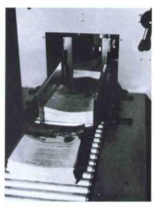
Completed, balanced and neatly jogged lifts move into the delivery area for stacking on skids, packing in boxes or conveying to a tying or shrink-wrapping machine without further handling.
